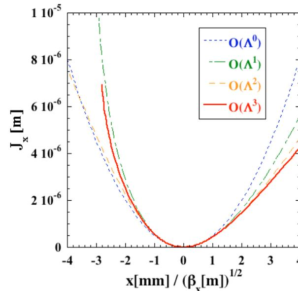
The relation between the action  $J_x$  and coordinate  $x$  is distorted at large amplitudes, and a naive lowest order treatment is inadequate.
